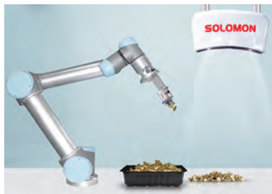
Bin pick robot with 3-D vision
