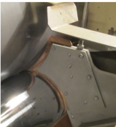
New Glue Dam with Absolute Position Feedback
