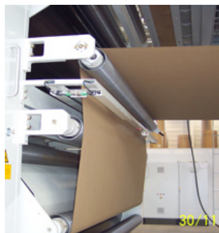
BHS LightGrid Technology for Paper Position Sensing
